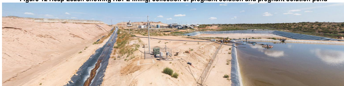
Figure 12 Heap Leach showing HDPE lining, collection of pregnant solution and pregnant solution pond
